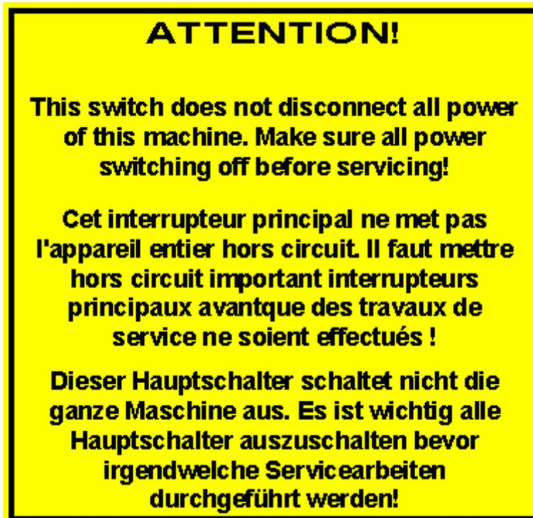
Illustration 13: This switch does not disconnect all power of this machine
