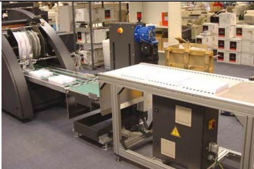
Pile Lift and roller table
