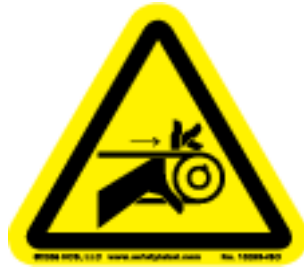
Illustration 7: Danger of entanglement from belt drive
